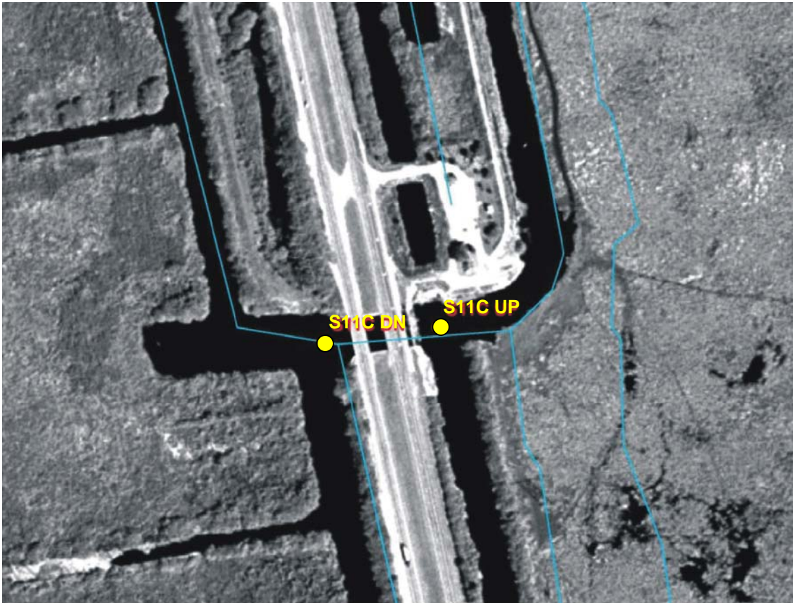
Figure 3. Example of head (UP) and tail (DN) gaging stations at S-11C. S-11C is a control structure in the levee dividing Water Conservation Area 2A from Water Conservation Area 3A-North.
