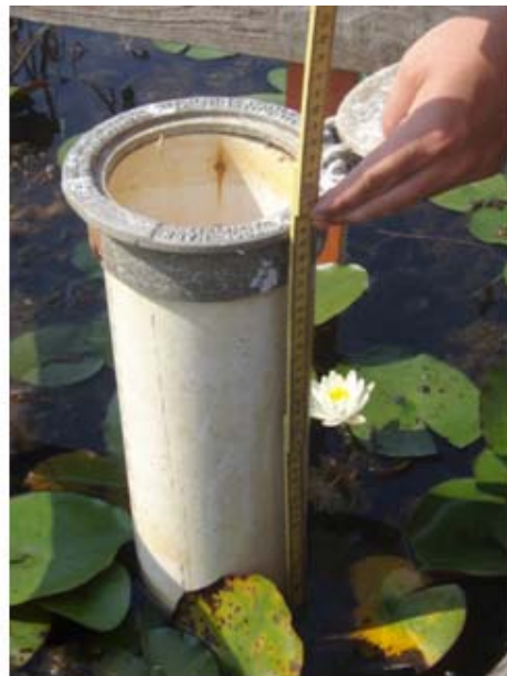
Figure 7. Illustration of how water-surface elevation measurements were made at FDEP elevation benchmarks.
